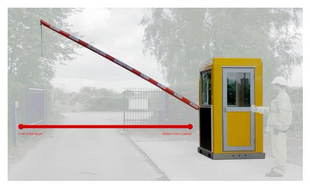
Should the closing barrier arm make contact with an obstruction not detected by the laser sensor, the previously described encoder in the motor will detect this. The motor will stop, reverse direction and return to the vertical open position. The barrier will exert a maximum force of 178N, less than the maximum force of 400N detailed in the BS-EN12445 and BS-EN12453 British Safety Standards.
